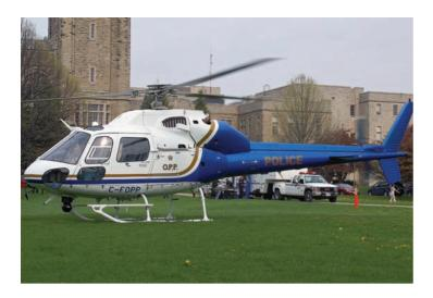
To increase performance and improve the Eurocopter AS355 operating characteristics, Eurocopter and Rolls-Royce designed a Supplemental Type Certificate (STC) to integrate the Rolls-Royce Model 250-C20R engine into F1 & F2 models of the AS355.
